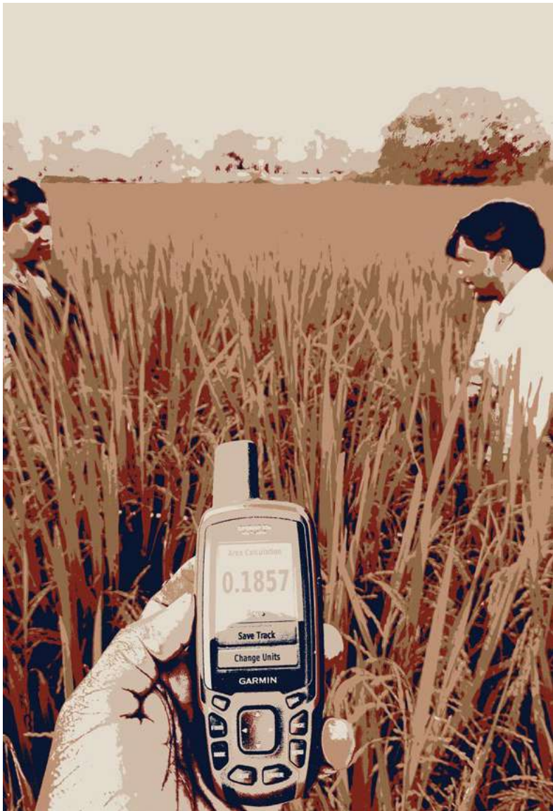
Fig 3.5, Using a GPS device to measure land area and capture geographic coordinates for accurate field measurement. This helps in precise estimation of crop area, yield calculation, and documentation of yield changes resulting from the adoption of improved agricultural practices.
